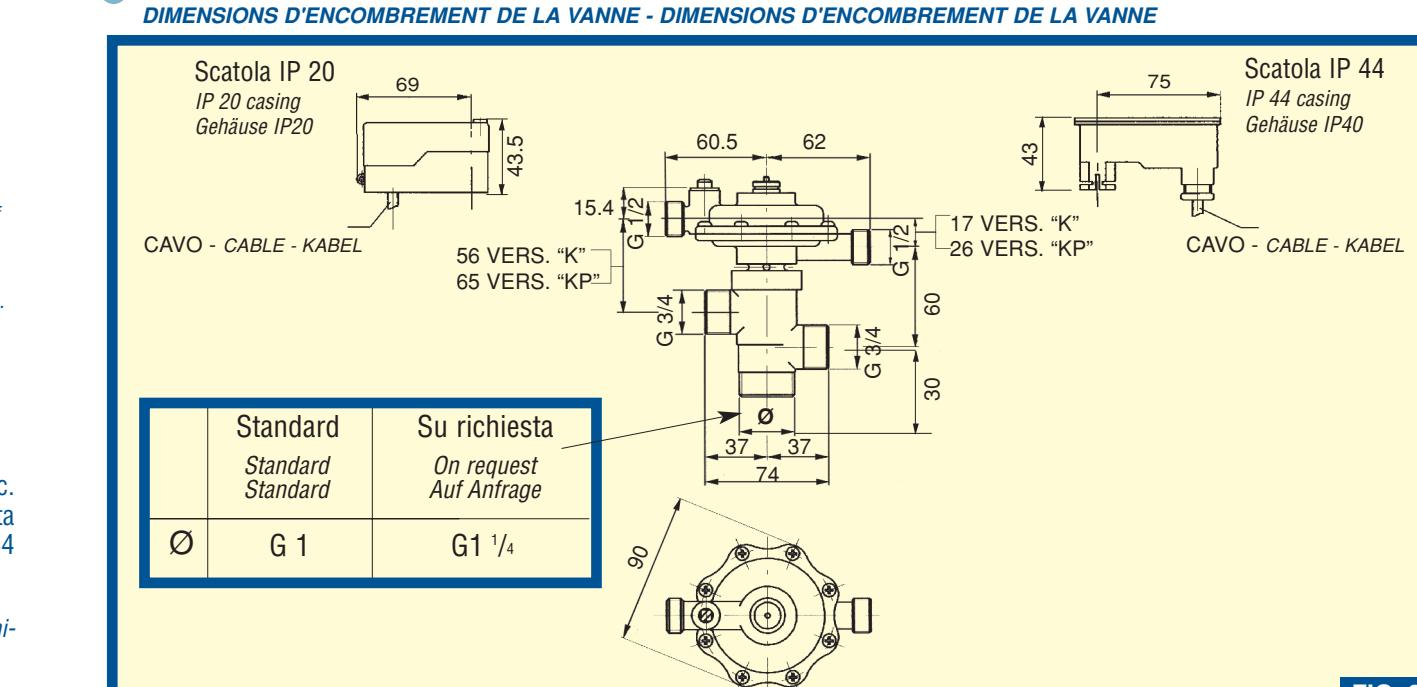
DIMENSIONI DI INGOMBRO GRUPPO SECONDARIO - OVERALL DIMENSIONS OF SECONDARY UNIT - ABMESSUNGEN SEKUNDÄRGRUPPE
