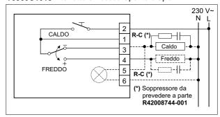
T6360C1000 Fan-Coil Caldo/Freddo, Commut. Est/Inv. Con Valvole V4043/V4044, M100+V58..4XXX
